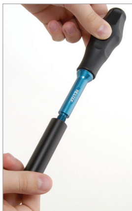
Screw the appropriate size attachment onto the end of the 2-in-1 Filter/O-Ring Insertion Tool Handle.
