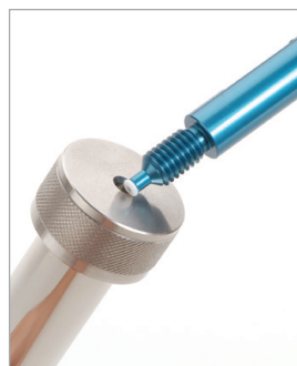
Insert the tool into the center hole of the extraction cell cap.
